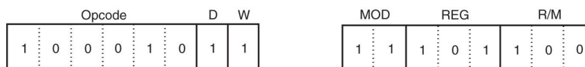
Figure 4-4 The 8BEC instruction placed into bytes 1 and 2 formats from Figures 4-2 and 4-3. This instruction is a MOV BP,SP.
